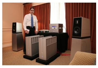
The biggest amps at the show and definitely some of the biggest in the world, Ypsilon Electronic's SET 100 amps aren't your garden variety solid state monsters. The Ypsilons put out only 120 watts of hybrid power with tubes in the input stage and mosfets for the juice. Like the name SET-100 implies, the amps are completely single ended. When you go for single ended in solid state, the amps gotta be huge.
