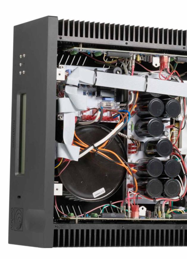
Considering the numerous components, it's difficult to criticize the Phaethon for not containing a full complement of point-to-point wiring. In our test model, the Silver Edition, silver wiring is used, as well as a special annealed material in the transformer windings.
